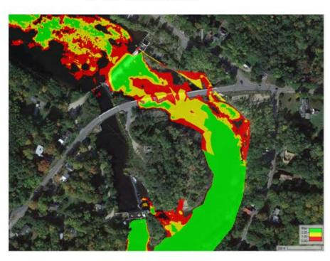
Figure 3 Water Depths at 762 cfs
