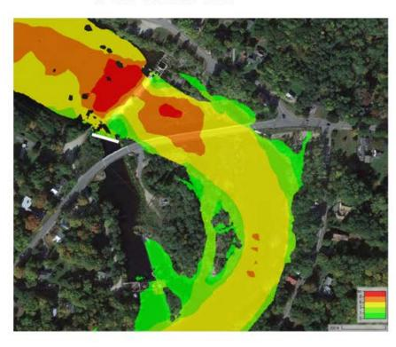
Figure 4 Water Velocities at 9,900 cfs
