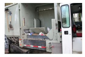
This body is divided into two separate compartments; it is called a 40/60 split. On this particular body the 40% side is located closest to the ditch side of the road. This happens to be the recycle side of the truck. The driver picks up the container with the recyclables that you have placed at curbside. See page two. Truck
